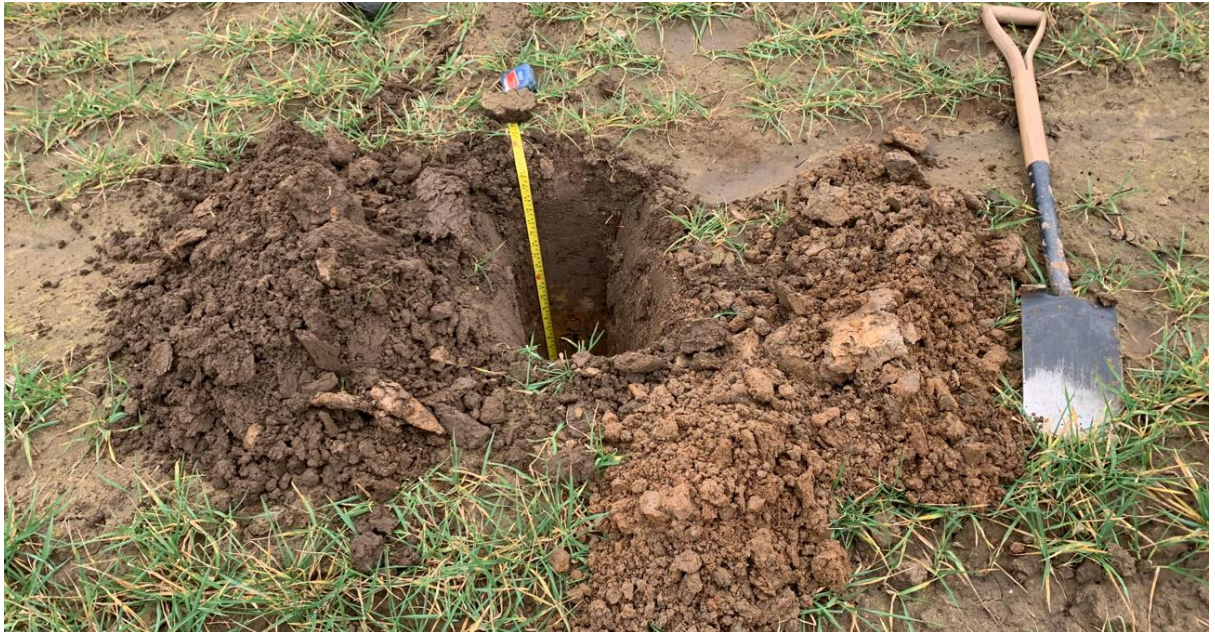
Photograph 14.14: Example Topsoil and Subsoil Colours (Photograph taken of soil examination in Field 34 of the Site)
